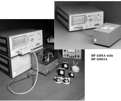
High Current Bias For Inductor Testing Under Load
