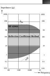
Impedance range (10% accuracy) comparison between HP 4286A versus reflections coefficient method
